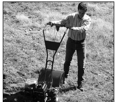
Fig. 4-5: With tines out of ground, push handlebars sideways to turn tiller.
